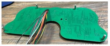
Step 4 Place the 3/8" Nylon spacers on the 1" screws
