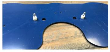
Attach overlay to the front of the circuit board using 4 #8-32 X 3/8" screws
