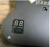
Step 3 Place the 2 #10-32 X 1" screws through the acrylic \*Make sure to remove protective film before install\*
