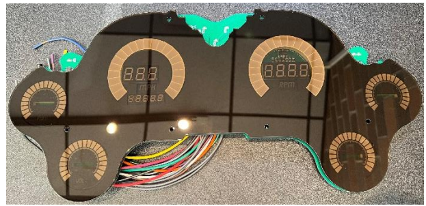
Place Acrylic over circuit board and overlay
