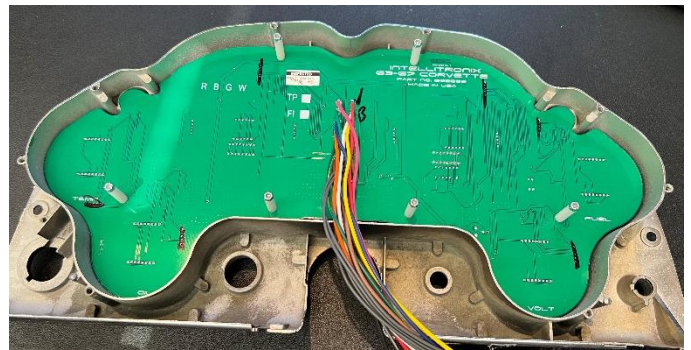
Insert circuit board assembly into housing
