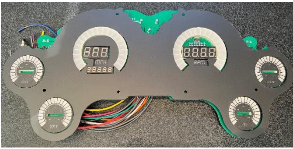
Place overlay on top of the gauges
