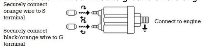
**Boost Gauge – Brown/Yellow.** Replace the existing Boost pressure sending unit with the sender included in the kit. The boost sender has two connections, one is for a ground connection marked G and the other is for the signal wire coming from the dash, marked WK.
