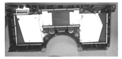
5. Remove the stencils and rubber blocks from the edges of the LED displays.
