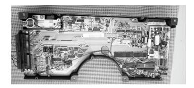
4. Remove the twenty-two (22) 7/32" screws securing the Display Driver Board of the gauge unit.
