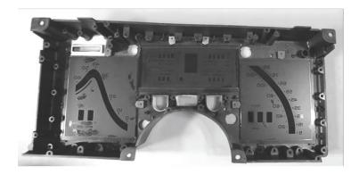
6. Remove the six (6) rubber clips securing the lenses.
