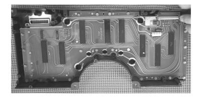
3. Remove the seven (7) 7/32" screws holding the Logic Board to the gauge unit.
