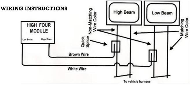
*Note: Automotive circuit connectors are the preferred method of connecting wires, although you may solder if you prefer.*
