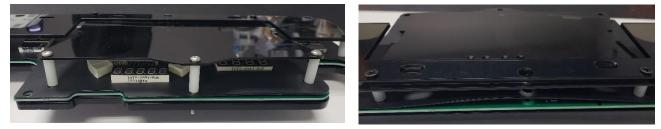
4. Attach the acrylic lens panel using 2 1 <sup>1</sup>/<sub>4</sub> " screws with 3/8" spacers at the top of the lens and the the 1 <sup>1</sup>/<sub>2</sub> " screws with <sup>3</sup>/<sub>4</sub>" spacer at the bottom of the panel as demonstrated in the above pictures. Secure all screws with a nylon washer and locking nut on the back of the assembly.
