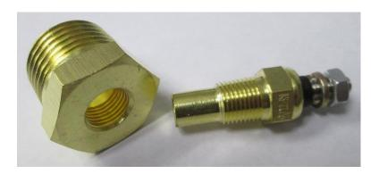
This sending unit may be used with our M9013 Water Temp Gauge; M9108 Oil Temp Gauge or M9107 Transmission Temp Gauge. It is supplied with an optional bushing. The wire from your selected gauge should be connected to the terminal at the top of the sender.
