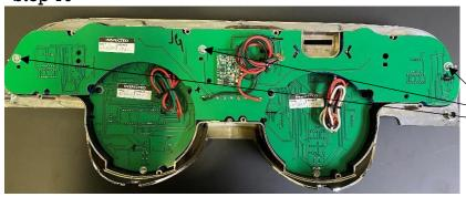
Insert the 3 #6 X 1" panhead screws to secure the instrument board into place
