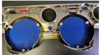
Place the #10 X 3/8" spacers over the screw holes as shown Step 4
