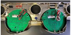
Insert the #6 X 1 <sup>1</sup>/<sub>4</sub> " panhead screws into the 4 locations with the washers 2 DP7002
