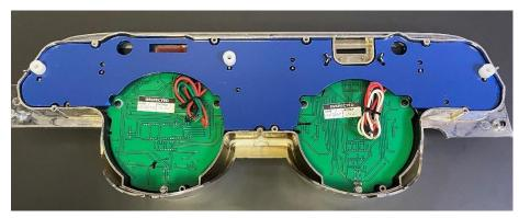
Use the #10 X 5/16" spacers between the lens and circuit board, following the locations pictured
