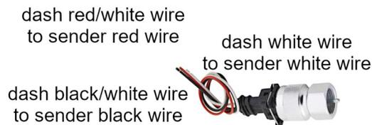
**!** If working with a factory VSS or computer-based engine you will NOT use the black/white or red/white wires.
