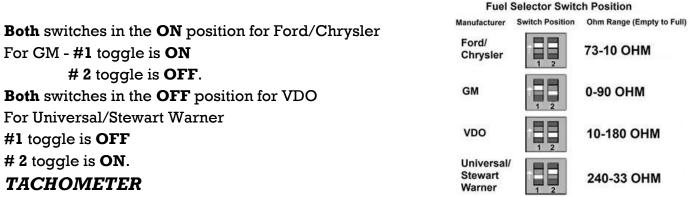
Note: If doing a LS engine swap, pick up the tach signal wire from the ECM/ECU and then set the tach switch to 4-cylinders. You may also need to order the Intellitronix LS Engine Swap Adapter Kit – for Series 1, 2 and 3 engines. The part number is 8014LS. If you are getting the tach signal from the ECU, the resistor in the adapter kit will help pull a stronger signal for the tachometer.
