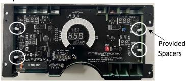
Remove factory gauges and insert the digital circuit board into the factory housing. Place provided spacers over existing screw holes
