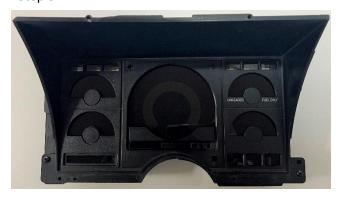
Place the factory bezel over the assembly and secure using the factory hardware. Now you can mount back into the vehicle.
