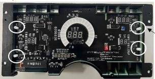
Remove factory gauges and insert the digital circuit board into the factory housing. Place provided spacers over existing screw holes
